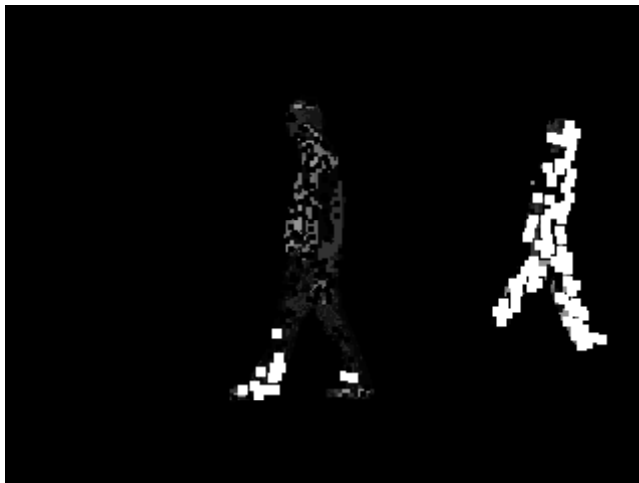
Backprojection person.1 using color and motion features
